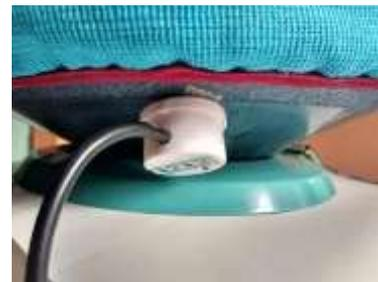
Gambar 5.1 Letak *Non-Contact Liquid Level Sensor*
